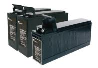
The rechargeable batteries are lead-lead dioxide systems. The dilute sulfuric acid electrolyte is absorbed by separators and plates and thus immobilized. Should the battery be accidentally overcharged producing hydrogen and oxygen, special one-way valves allow the gases to escape thus avoiding excessive pressure build-up. Otherwise, the battery is completely sealed and is, therefore, maintenance-free, leak proof and usable in any position.
