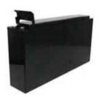
The rechargeable batteries are lead-lead dioxide systems. The dilute sulfuric acid electrolyte is absorbed by separators and plates and thus immobilized. Should the battery be accidentally overcharged producing hydrogen and oxygen, special oneway valves allow the gases to escape thus avoiding excessive pressure build-up. Otherwise, the battery is completely sealed and is, therefore, maintenance-free, leak proof and usable in any position.
